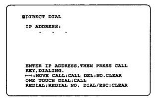
2. Press the REDIAL button. The dialog screen displays the IP address that has been the latest dialing.
