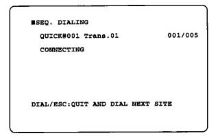
The sequential dialing starts to let the Control site view the images sequentially. The sequence will skip to the next when the called site is busy or does not respond for more than 150 seconds.
