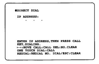
Press a one-touch dial button. The dialog screen changes to "CONNECTING" and the unit starts dialing.
