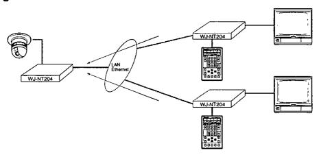
There are some limitations on the right of control when more than one WJ-NT204 receiver (Control site) access to one transmitter (Remote site).
