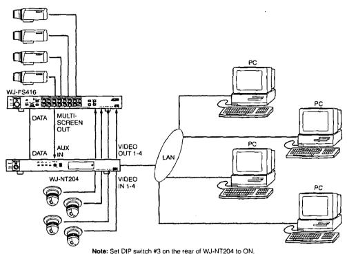
Note: Set DIP Switch #3 on the rear of WJ-N1204 to Or
