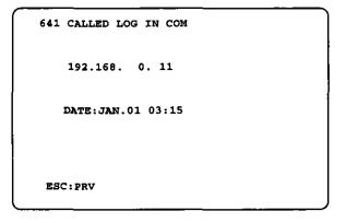
You can check the registered name and address, and received date and time on the monitor. This log will be lost when the unit is turned off the power.
